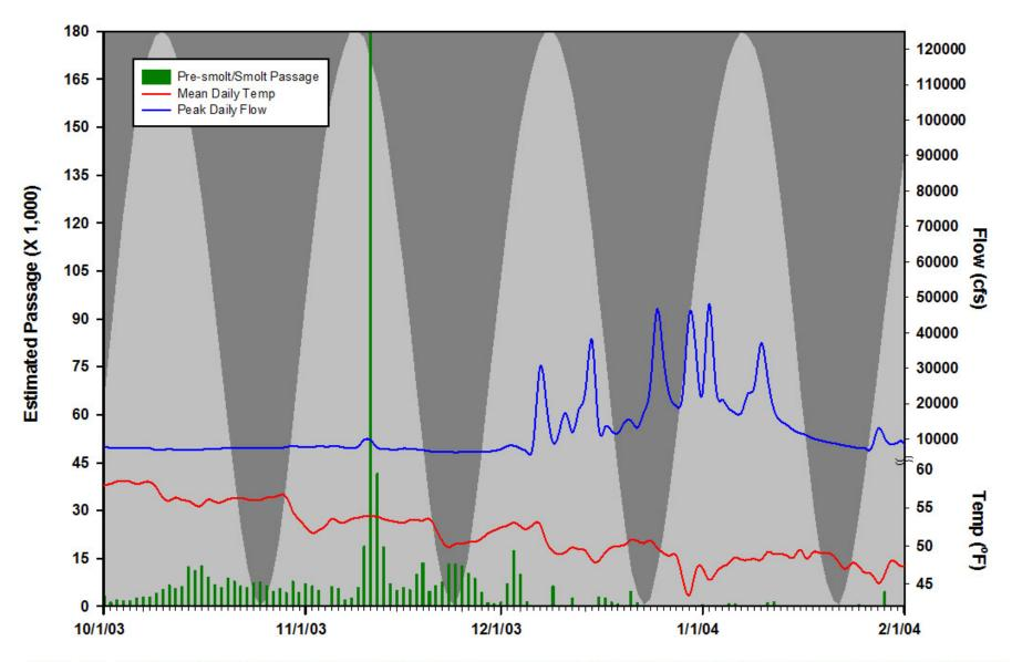
Figure A13. Brood Year 2003 winter Chinook pre-smolt/smolt passage with moon illuminosity indicated by back ground shading (peak of light gray equals full moon), mean daily water temperatures (red), and peak daily flows (blue) at Red Bluff Diversion Dam.
