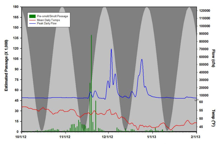
Figure A22. Brood Year 2012 winter Chinook pre-smolt/smolt passage with moon illuminosity indicated by back ground shading (peak of light gray equals full moon), mean daily water temperatures (red), and peak daily flows (blue) at Red Bluff Diversion Dam.
