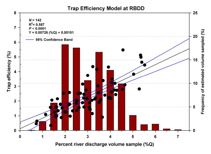
Figure 3. Trap efficiency model for combined 8-ft diameter rotary traps at Red Bluff Diversion Dam (RM 243), Sacramento River, CA. Mark-recapture trials (N = 142) were used to estimate trap efficiencies. Histogram indicates percentage of time traps sampled various levels (half percent bins) of river discharge between April 2002 and September 2013.
