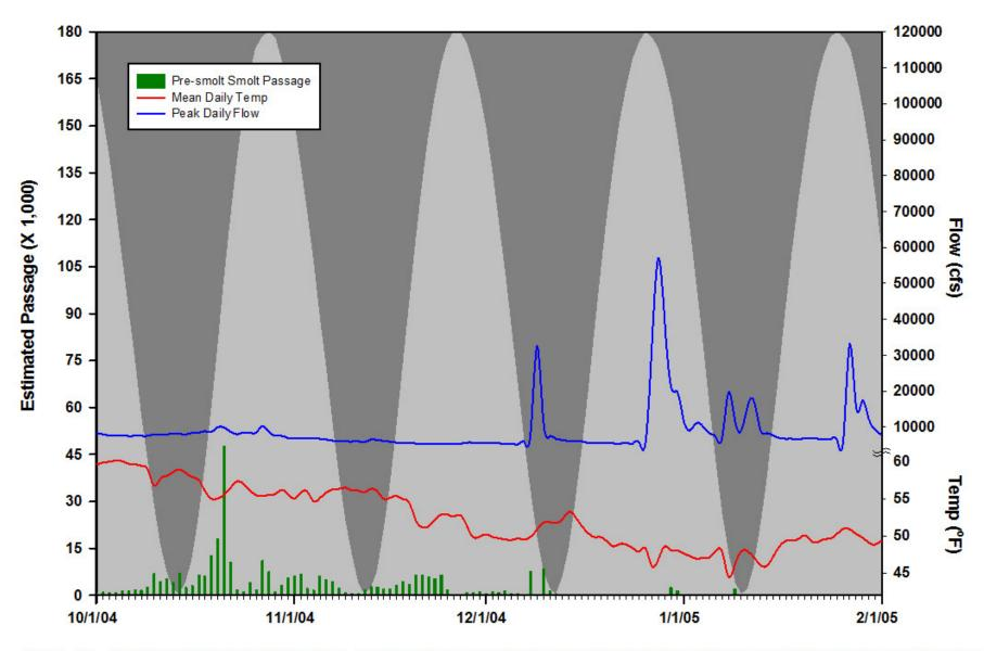
Figure A14. Brood Year 2004 winter Chinook pre-smolt/smolt passage with moon illuminosity indicated by back ground shading (peak of light gray equals full moon), mean daily water temperatures (red), and peak daily flows (blue) at Red Bluff Diversion Dam.
